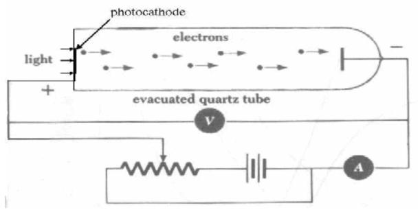
(c) Using the apparatus above scientists can measure the stopping voltage needed to stop the photoelectrons causing a current. Draw a graph of stopping voltage against frequency and show what measurement can be used to determine the energy needed to ionize the photocathode.
